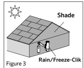
Once the Rain-Clik is mounted, run the wire to the controller, and fasten it every few feet with wire clips or staples for best results. Be careful not to cut through the wire insulation with fastening hardware or chaff the insulation when routing wire through or around metal materials (e.g., gutter, siding, etc.). If an extension to the wire provided is needed, use the following table to determine the minimum wire gauge needed:
