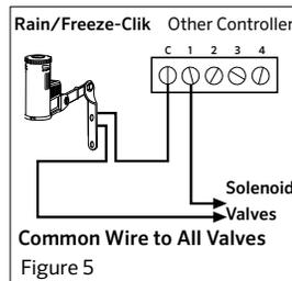
**Note:** The common wire to the valves does not have to be interrupted at the controller. The Rain-Clik can be wired anywhere along the common wire line.
